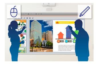
Connecting the projector to a PC via USB cable makes it possible to operate the PC mouse using the included interactive pen and even your finger.
