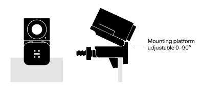
Screen Mount with camera on top of display
